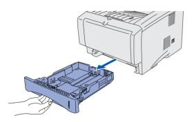
While pressing the paper guide release lever, slide the adjusters to fit the paper size. Check that the guides are firmly in the slots.
